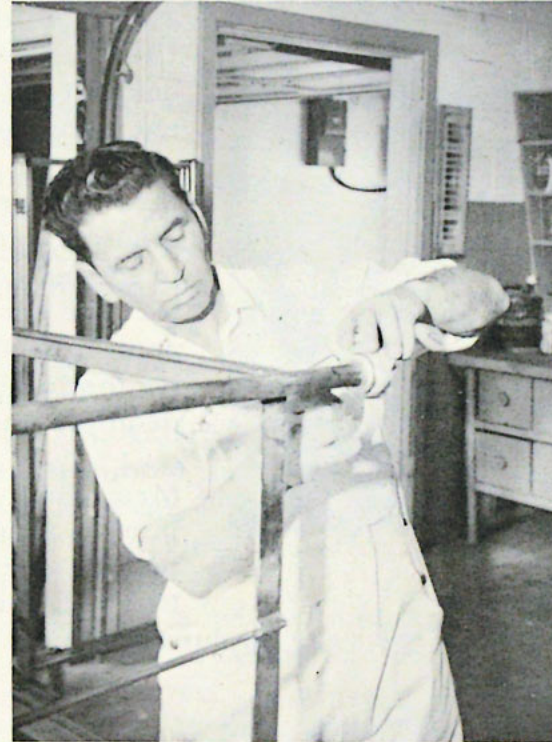
2. With almost every item to be refinished, disassembling is the first step in the refinishing process. Casters, knobs, shelves, upholstered pads, must all be removed. Above, Don Rau removes casters from a portable cart.
