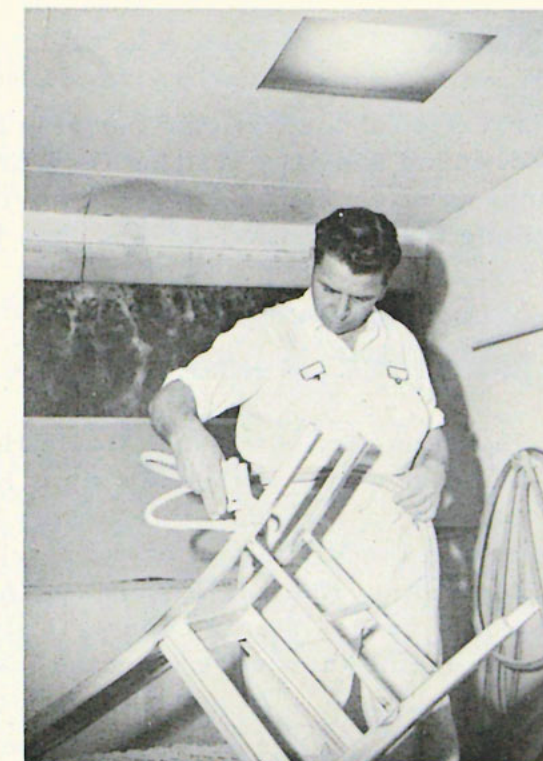
5. In the spray booth, a chair gets a fresh coat of paint. A 36-inch exhaust fan draws off almost all paint mist in the air through a filtering waterfall bath visible in the background of the picture above. Masks must be worn when enclosed areas, such as inside of cabinets, are being sprayed.
