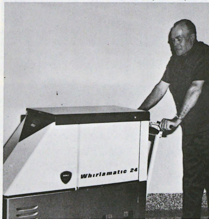
THEODORE KUKLOK, PORTER, IS SHOWN OPERATING THE NEW SCRUBBER RECENTLY PURCHASED FOR THE HOUSE-KEEPING DEPARTMENT FOR USE IN THE NEW WING. THE "WHIRLMATIC 24" SWEEPS, CLEANS AND WAXES IN ONE OPERATION, POWERED BY FOUR 6-VOLT BATTERIES. THE SELF-CONTAINED UNIT NEEDS NO ELECTRIC CORDS, AND BATTERIES ARE RE-CHARGED DAILY FOLLOWING USE.
