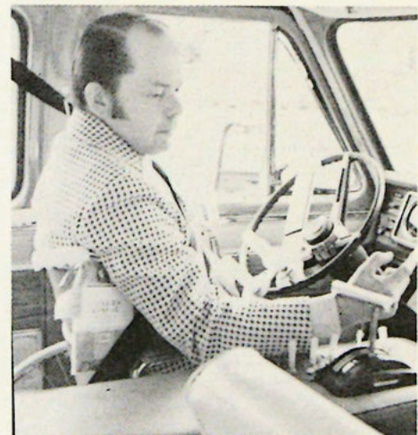
A representative from the Redi-Care Company demonstrates the use of the power automatic transmission in the Quadrapelegic Van.
