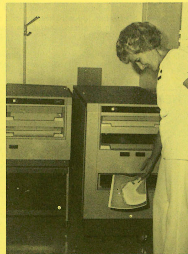
LEFT: Radiologic Technologist, Mary Pikus, uses a new x-ray imaging system recently added to SCH's Department of Radiology. The new system is known as xeroradiography and has been developed by the Xerox Corporation. It is used with present x-ray equipment and represents a new concept in recording high quality x-ray images on paper. This eliminates the need for conventional x-ray film and a darkroom. This equipment is used primarily for mammography (x-ray examinations of the female breast) at SCH.
